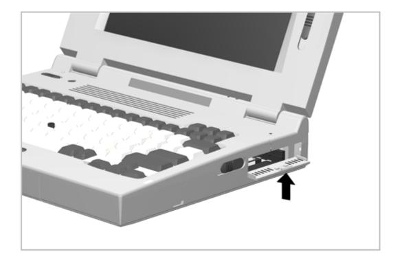
Figure 5-21. Removing the PC Card Door
